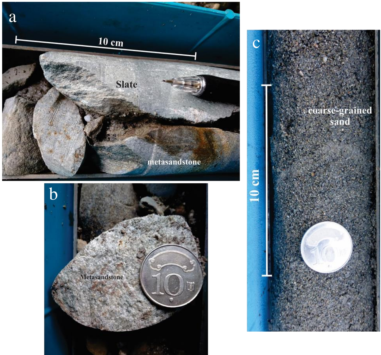
Figure 3.9 Close view of alluvium sourced from the Central Range (AlCeR). (a) Rock core of DP-8 at depth 29.8 – 30 m. (b) Metasandstone of AlCeR. (c) Rock core of DP-7B at depth 44.3 – 44.4 m.
