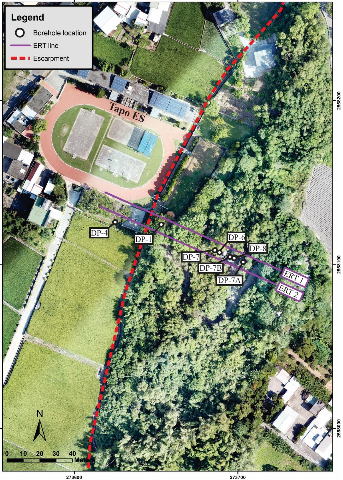
Figure 2.1 Bird view image of research area along with configuration of Electric Resistivity Tomography (ERT) survey line and boreholes.
