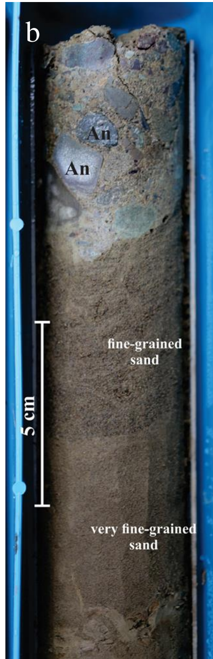
Figure 3.8 Close view of alluvium sourced from the Costal Range (AlCoR). Label “An” indicates the andesitic pebble. (a) Rock core of DP-7B at depth 15.5 – 16.5 m. (b) Rock core of DP-1 at depth 12– 12.3 m.
