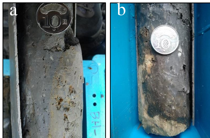
Figure 4.2 Photograph of the lithologic contact between the mud and the Holocene sediment. (a) Photograph of lithological contact between mud (left side) and fine-grained sand (right side) on borehole core 7B at depth of 16 m. (b) Photograph of lithological contact between sand (left side) and mud (right side) on borehole core 8 at depth 28 m.
